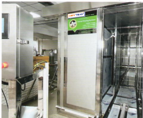
Conveying tunnel drying system, batch feeding and discharging.
