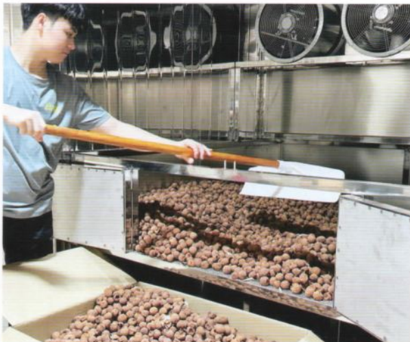
Customized dryer and software for cardamom drying with preset program to simplify operation.
